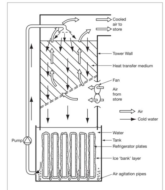
Fig 28 Ice bank cooler construction
