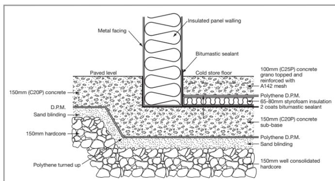
Fig 33 Floor construction and panel bottom
