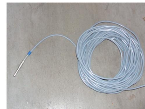
Fig 36 Typical temperature probe used to monitor temperature of air or produce within a cold store
