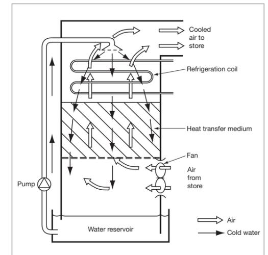
Fig 27 Spray chill cooler construction
